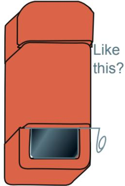
At fig. 7, there is a damper made out of stainless sheet metal. See the detail photos for a good view: the hinge is a bit of wire running L to R along the upper side. The sheet metal wraps around the wire. The L end of the wire makes a pin which sits on the brick. The R side goes through the brick to make the handle, which is bent into a spiral.
