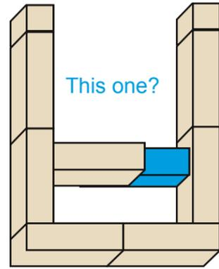
in 2a, the left hand brick in the upper horizontal course is short, allowing gases in the oven bell to move around and up (this is barely visible in the video).
